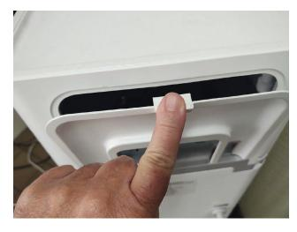
2. Slightly pull the Top cover back from over the tabs on the back corners of the unit.
