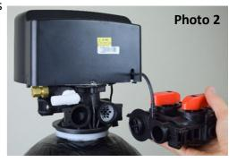
side the flow meter assembly (the piece with the cable attached) is still connected to. If the piece with the cable is still attached to the valve head, use a small flathead screwdriver to pry the flow meter piece apart (Picture 2)
